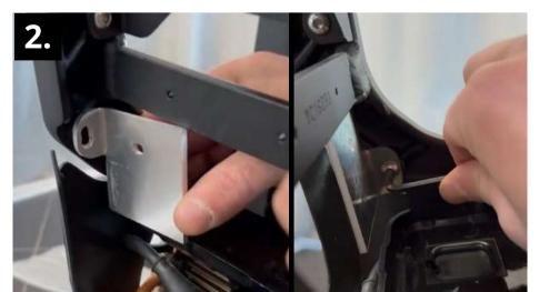
STEP 2: Fasten the brackets to the each side of the bike frame using these bolts:
