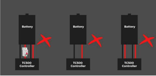
Use only tools and screws that came with the controller. Using the tools and screws that were not included in the parcel, not following these instructions, or not using the circuit breaker, will void your 2-year warranty and can cause serious damage to you and your bike, and voids your 2-year warranty.
