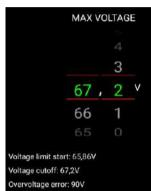
Max Voltage affects the regen. If the voltage of the battery is between the "Voltage limit start" value and the "Voltage cutoff" value, the regen is reduced. If the voltage of the battery is above the "Voltage cutoff", the regen is automatically disabled. If the battery voltage is above 90V, the "Overvoltage error" is displayed and the bike stops.
