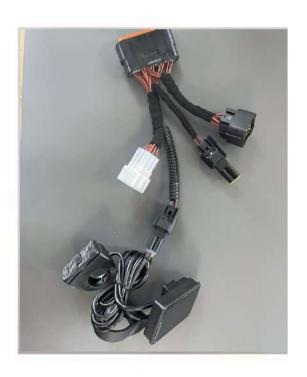
The Torp display is being installed directly to the controller's wiring harness, as shown on the photos.
