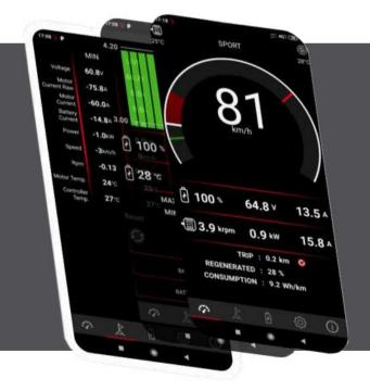
All the settings and diagnostics are managed through an intuitive and easy-to use smartphone app for Android and IOS. The users can use their smart-phone as a display during the rides and to set up all the controller`s features through the app.
