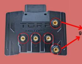
Don't apply silicone grease on the terminals or other parts of controller!
