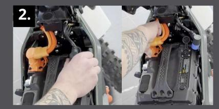
Now you can start removing the stock SurRon controller and lower the skid-plate that covers the wiring.
