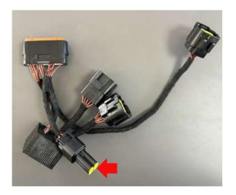
The Torp Display is being installed directly to the controller's wiring harness, as shown on the photo.
