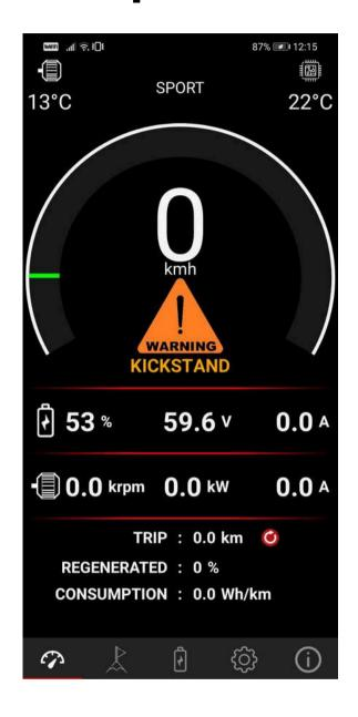
IMPORTANT: After the installation make sure to calibrate the throttle and Hall sensors! Go to the 5th screen of the Torp App and click the CALIBRATION button. Then follow the setup Wizard. CALIBRATION must be repeated after each firmware update!
