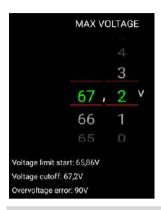
**9-Max Voltage:** Max Voltage affects the regen. If the voltage of the battery is between the "Voltage limit start" value and the "Voltage cutoff" value, the regen is reduced. If the voltage of the battery is above the "Voltage cutoff", the regen is automatically disabled. If the battery voltage is above 90V, the "Overvoltage error" is displayed and the bike stops.
