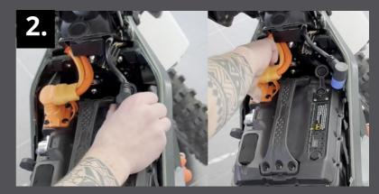
Now you can start removing the stock SurRon controller and lower the skid-plate that covers the wiring.
