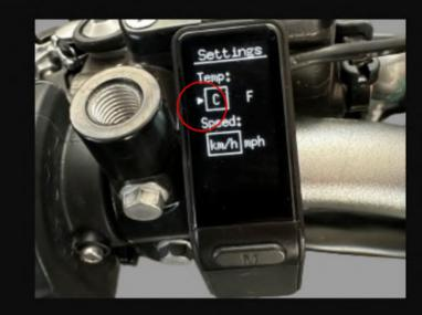
HOLDING THE SELECT/CHANGE BUTTON SWITCHES BETWEEN TEMPERATURE AND SPEED MEASUREMENT UNITS.
