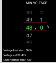
reached, the motor will stop and a UNDERVOLTAGE error will be displayed on the 1st screen of the App.
