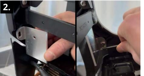
STEP 2: Fasten the brackets to the each side of the bike frame using these bolts:
