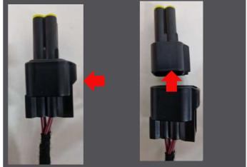
The Torp Display is being installed directly to the controller`s wiring harness, as shown on the photo.
