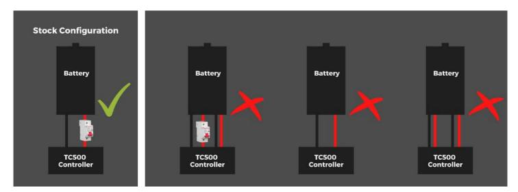
Use only tools and screws that came with the controller. Using the tools and screws that were not included in the parcel, not following these instructions, or not using the circuit breaker, will void your 2-year warranty and can cause serious damage to you and your bike, and voids your 2-year warranty..
