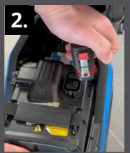
Now you can start removing the stock Talaria controller and the battery from the frame, and lower the skid-plate that covers the wiring.
