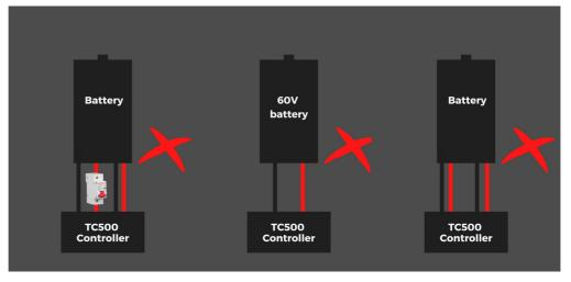
The TC1000 controller must always be used with a stock SurRon/Segway circuit breaker (fuse)! Not using the circuit breaker with controllers is dangerous and can cause serious damage!
